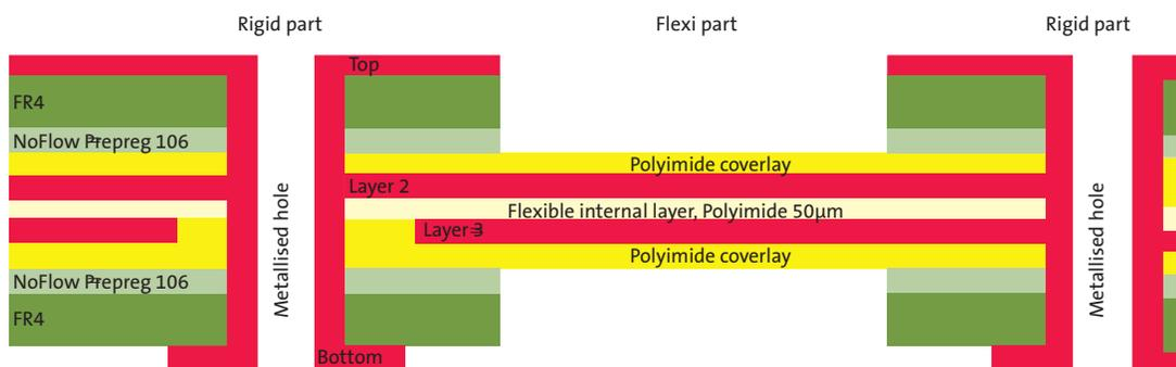
Abb. 2: Example structure of a 4 layer multilayer board with a flexible internal layer
