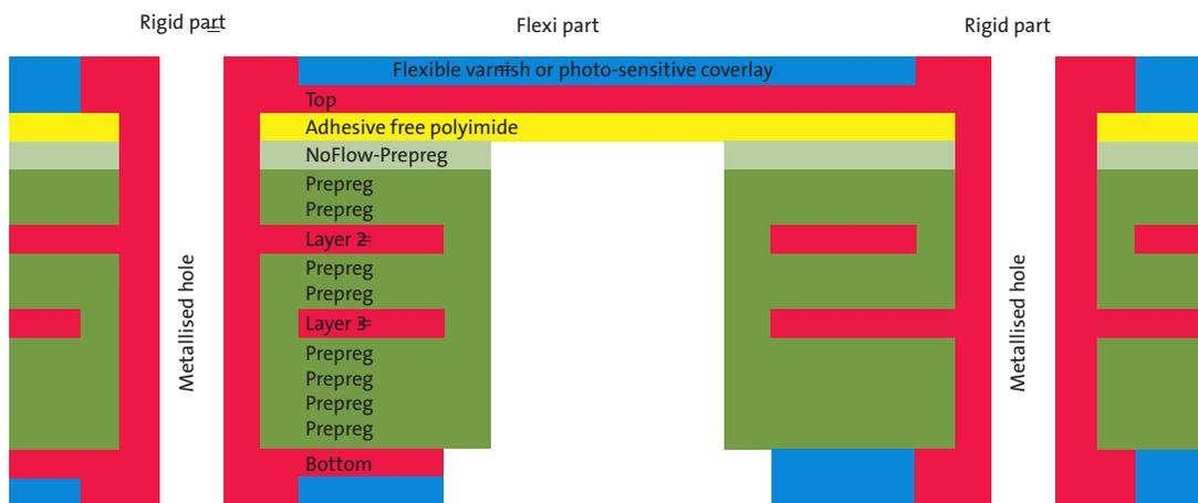
Abb. 1: Example structure of a 4 layer board with a flexible top layer
