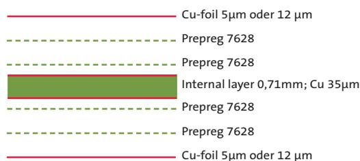
**Standard structure 6 layer multilayer, pressed thickness approx. 1.50 mm**
