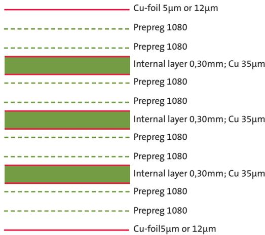
**Standard structure 10 layer multilayer, pressed thickness approx. 1.60 mm**
