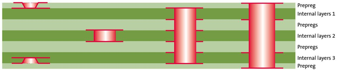
A  $1+(1+(4)b+1)+1$  SBU multilayer board which is pressed three times
